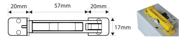
Mounting holes - 14mm from escutcheon cut out to centre of hole.
